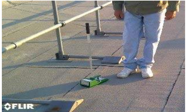
PHOTO 10 Upper Roof Section: Tramex meter was place on roof surface every 2-4 feet in grid pattern.
