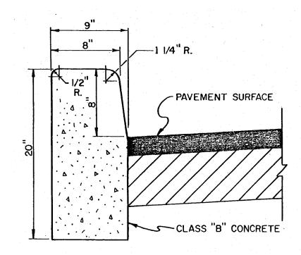
NOTE: TRANSVERSE JOINTS 1/2" WIDE SHALL BE INSTALLED 10'-0" APART & SHALL BE FILLED WITH PREFORMED BITUMINOUS JOINT FILLER AASHO DESIGNATION M 213 RECESSED 1/4" FROM TOP AND FACE. DEPRESSED CURB AT DRIVEWAYS PER 605.02, NJDOT STD SPEC. FOR ROAD AND BRIDGE CONSTRUCTION, 1989.
