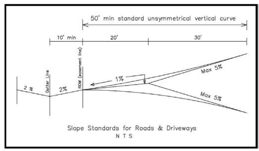
Note: The vertical curve portion of the diagram above also applies to driveways using a concrete apron.
